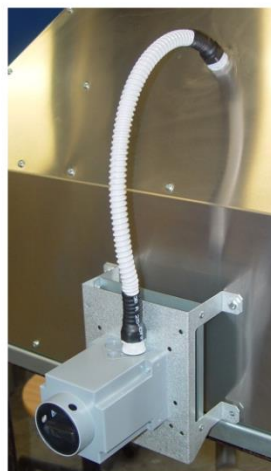
Properly mounted service switch, cable protected inside tube
