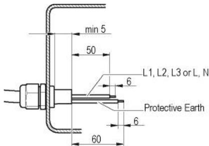
Only strip the cable as far as necessary, ensuring that the cable gland is sealed and there is no strain on the connections. For tightening torques, see Chapter 3.1 Product drawing.
